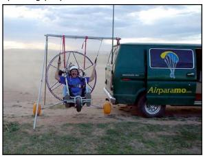
**WARNING:** Be extremely cautious to run the motor on the trike while it is being hang tested. If you do want to run up the motor in the hang test rig, be sure to do this in a secure, sturdy hang test rig and with the assistance of an experienced instructor who is thoroughly familiar with motor runups in a hang tester.
