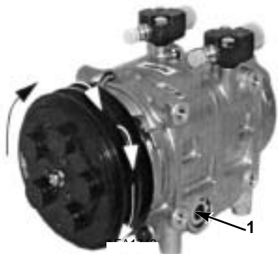
1. Compressor Oil Sight Glass
