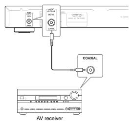
This enables you to listen to surround sound. For a coaxial connection, use a coaxial cable (supplied) to connect the "COAXIAL DIGITAL AUDIO OUT-PUT" jack to a coaxial input on your AV receiver.
