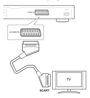
This connector can output composite video, or RGB video. The default setting is composite, which should work with all TVs. Consult the manual that came with your TV to see if you can use one of the higher quality settings. See page 42 for how to change the video output.
