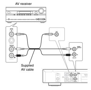
The diagram shows standard video connections, but you can alternatively use the component video connections if it's available.
