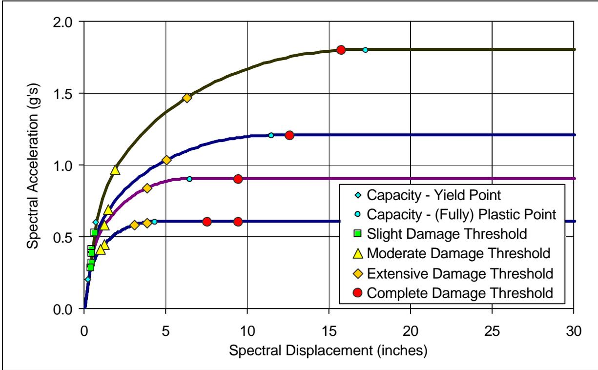
**Figure 2.7. Generic Building Type W1 (Light Frame Wood < 5,000 sq. ft.)<sup>1</sup> – Capacity Curves and Structural Damage-State Thresholds (Fragility Medians) for Five Seismic Design Levels (Special High, High, Moderate, Low and Pre-Code)**
