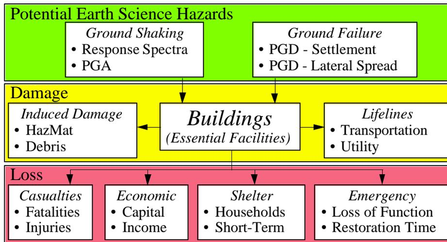
**Figure 2.1. Building-Related Modules of the FEMA/NIBS Methodology**
