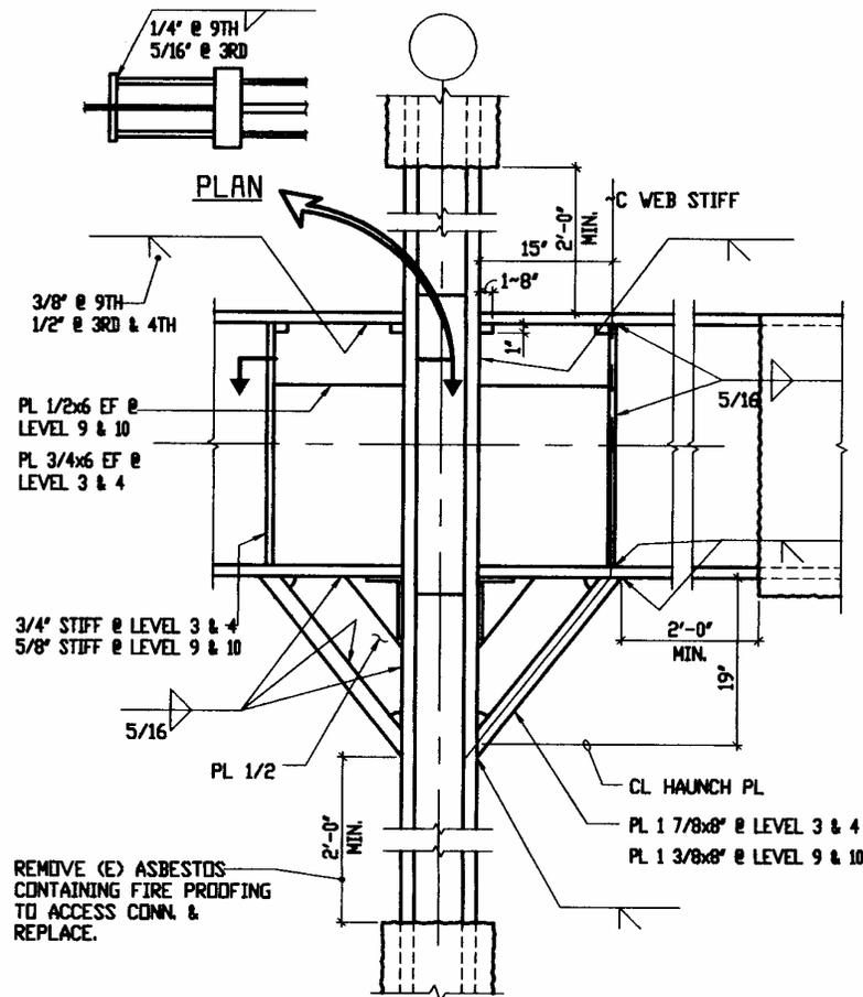
Figure 8.5. Typical Girder-Column Strengthening Detail [Chen et al., 2001]
