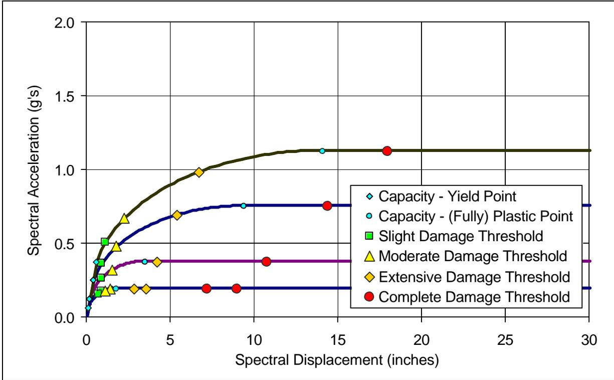
**Figure 2.9. Generic Building Type C1L (Low-Rise Concrete Moment Frame)<sup>1</sup> – Capacity Curves and Structural Damage-State Thresholds (Fragility Medians) for Five Seismic Design Levels (Special High, High, Moderate, Low and Pre-Code)**
