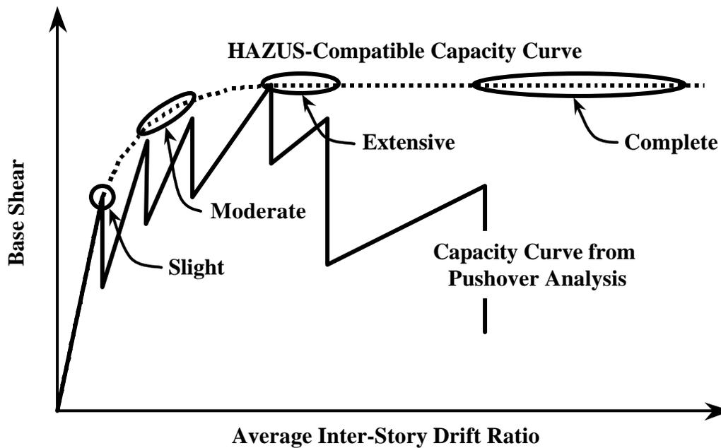
Figure 6.4. Example Damage-State Medians of "Saw-Tooth" Pushover Curve
