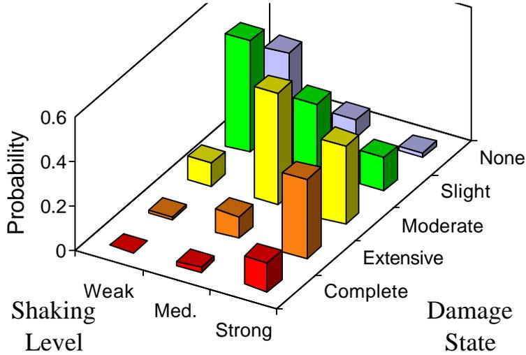
**Figure 2.6. Example Damage-State Probabilities for Weak, Medium and Strong Shaking Levels**
