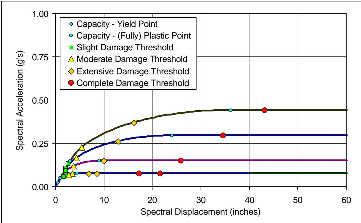
**Figure 2.11. Generic Building Type C1H (High-Rise Concrete Moment Frame)<sup>1</sup> – Capacity Curves and Structural Damage-State Thresholds (Fragility Medians) for Five Seismic Design Levels (Special High, High, Moderate, Low and Pre-Code)**
