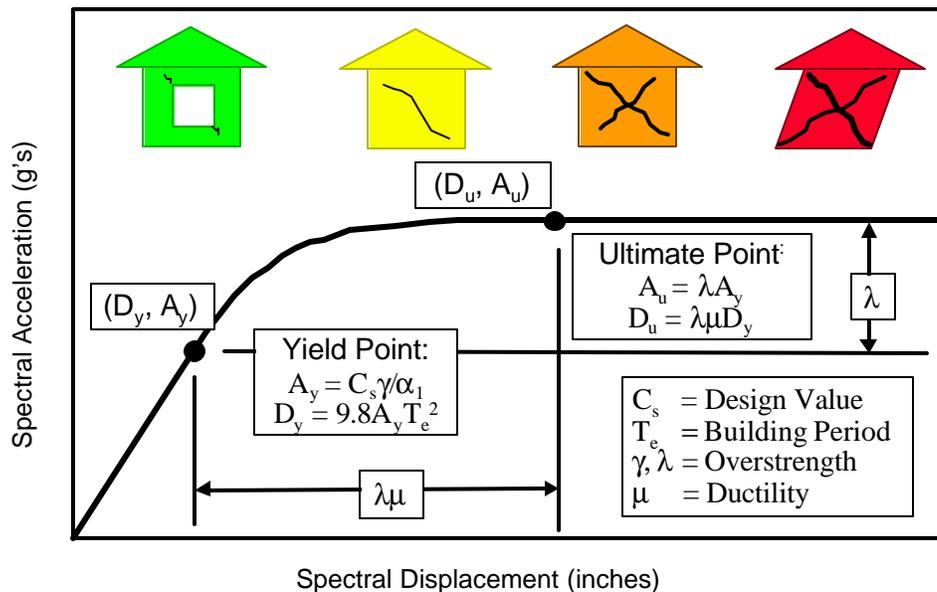
**Figure 2.3. Example Building Capacity Curve and Control Points**
