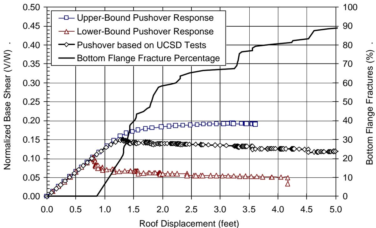
**Figure 8.6. Pushover Curves and Connection Damage – Original Building**
