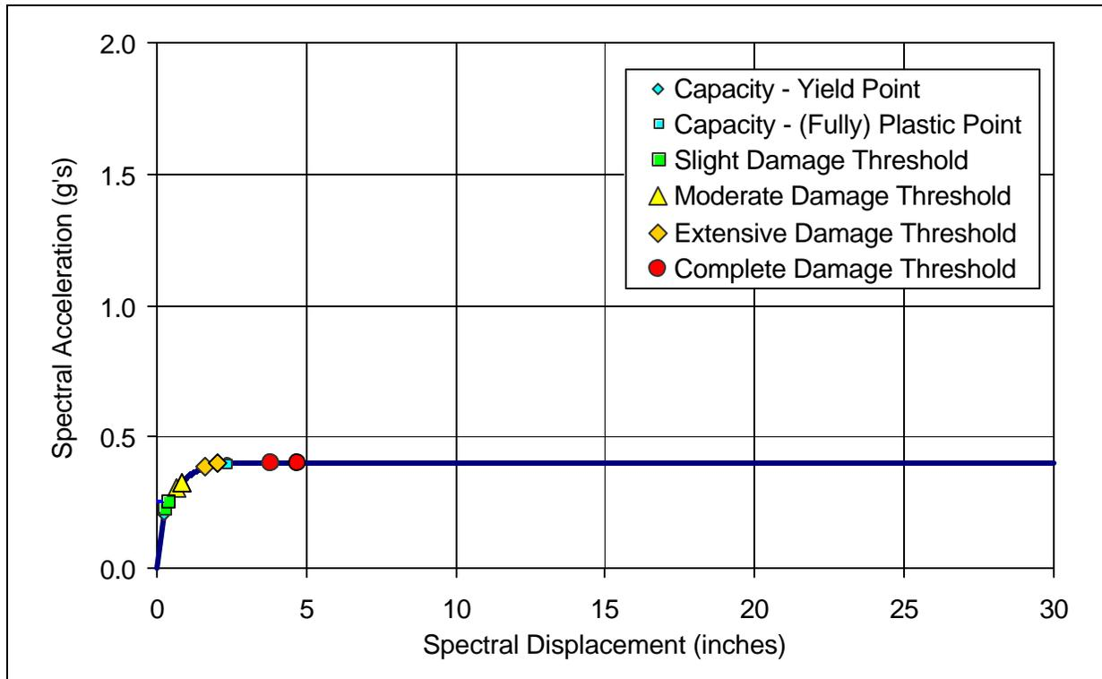
**Figure 2.8. Generic Building Type URML (Low-Rise Unreinforced Masonry Bearing Walls)<sup>1</sup> – Capacity Curves and Structural Damage-State Thresholds (Fragility Medians) for the Pre-Code Seismic Design Level**
