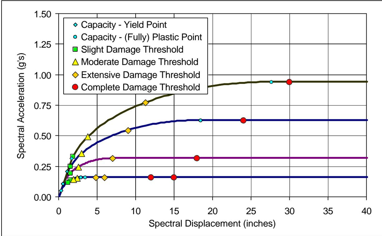
**Figure 2.10. Generic Building Type C1M (Mid-Rise Concrete Moment Frame)<sup>1</sup> – Capacity Curves and Structural Damage-State Thresholds (Fragility Medians) for Five Seismic Design Levels (Special High, High, Moderate, Low and Pre-Code)**
