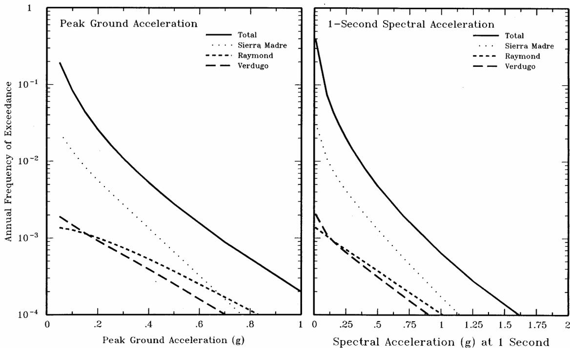
**Figure 8.8. DPW Building Site Hazard Curves [Geomatrix, 1999]**
