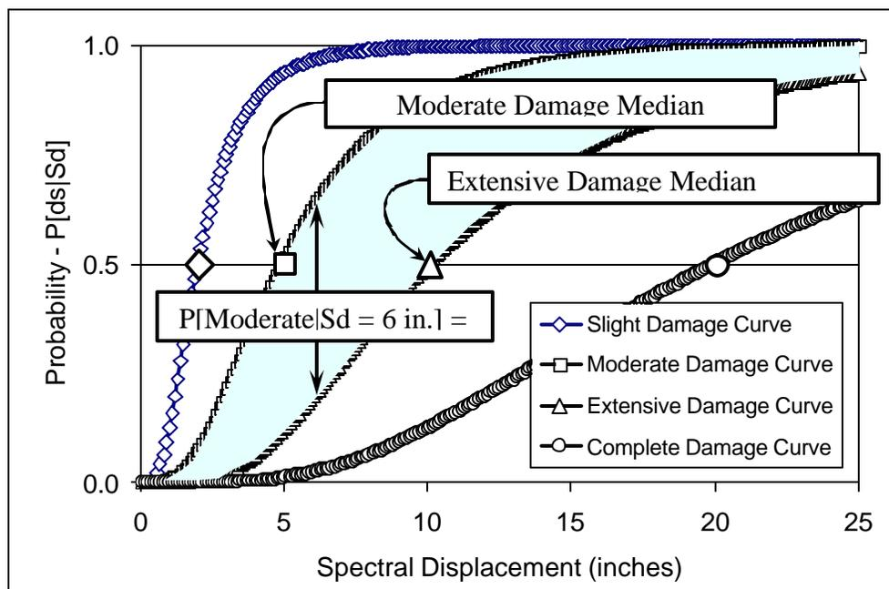
**Figure 6.1. Example Fragility Curves - Calculation of Damage-State Probability**
