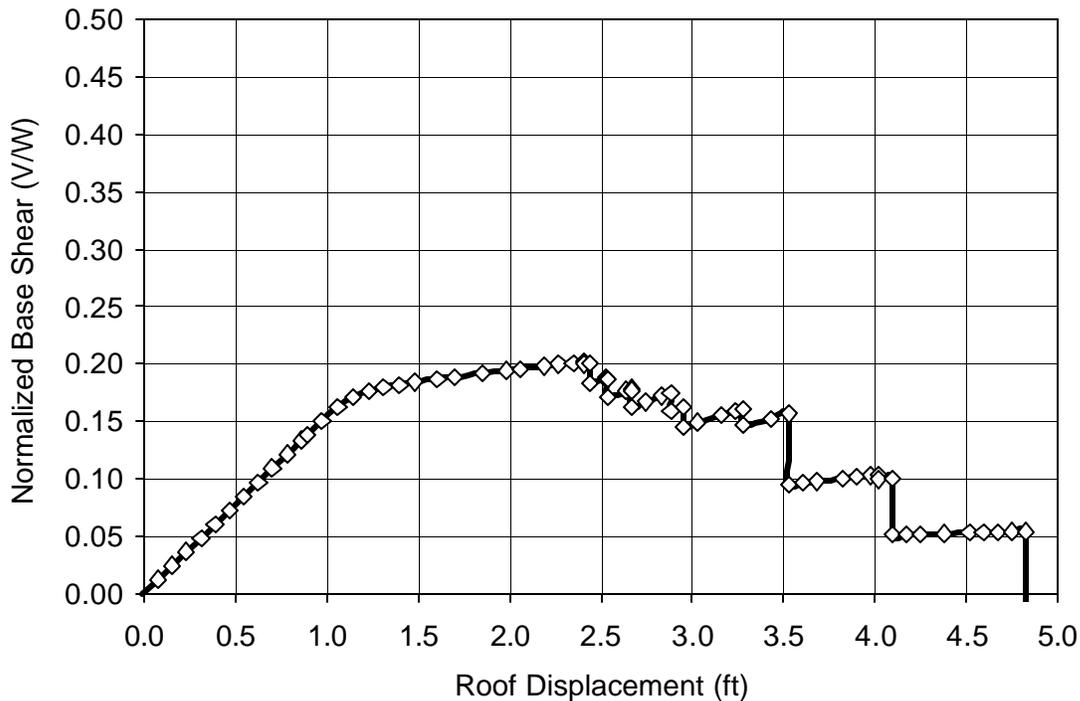
**Figure 8.7. Pushover Curve – Connection-Only Retrofit Scheme**
