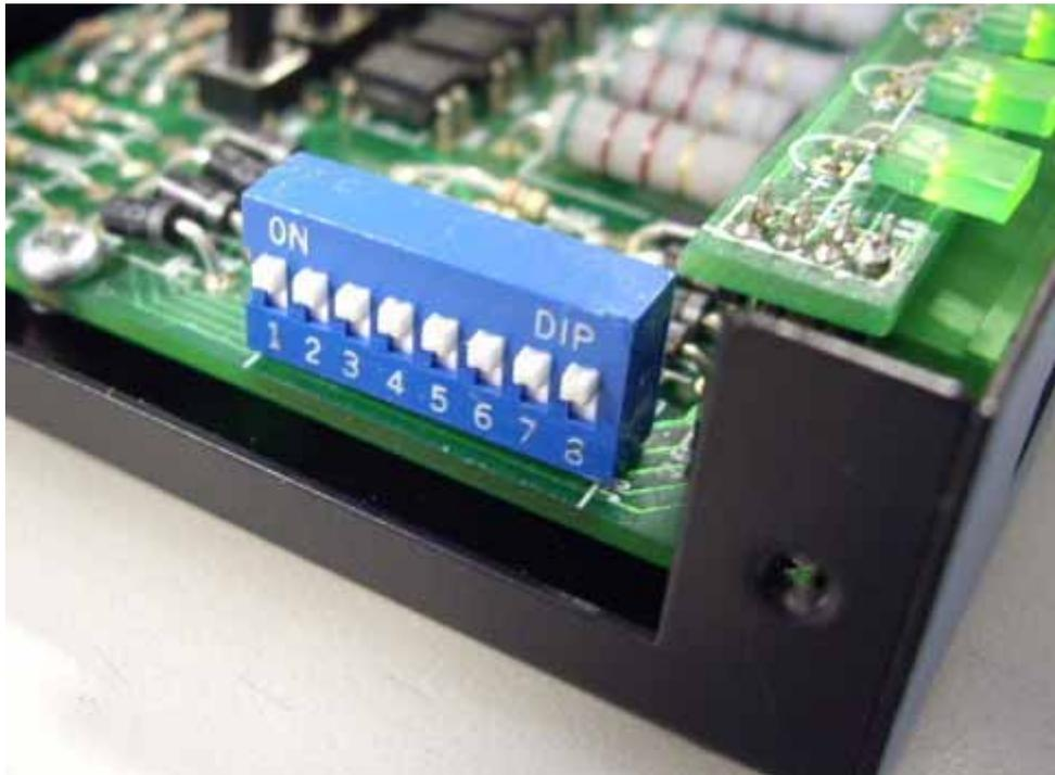
Then you can setup the Dry/Wet contact in left switch :
