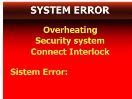
The system will then put itself automatically to a safe state: the laser source will be automatically deactivate as well as the foot switch (stand by state).
