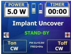
Bring the system to the "Stand-by" state pushing the "Stand By/Ready/Operate" button.
