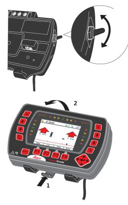
To turn the system on and off, use the power switch on the right side of the cradle. This is the master switch for the entire system.
