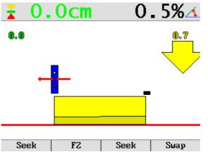
If both keys are pressed, and held for more than three seconds, the control panel will take the current sensor value and store as the new reference height.
