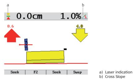
A cross slope is selected in the right side and in the left side a Laser Sensor is selected.
