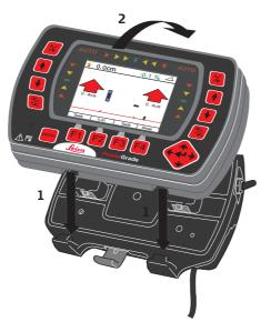
To connect the control panel to the cradle:
