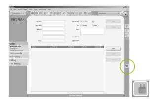
If no iCube has been previously connected, pressing the iCube status button will start the "Connection Wizard for iCube". (Later, pressing the iCube status button will guide you directly to the "CableFree Fitting Status" screen as described on page 18).
