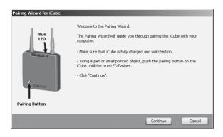
To initiate the pairing process on iCube, set the device into pairing mode by pressing and holding the Bluetooth pairing button for 2 seconds until the Bluetooth indicator is blue and flashing fast. iCube is now in pairing mode for two minutes or until pairing is completed.
