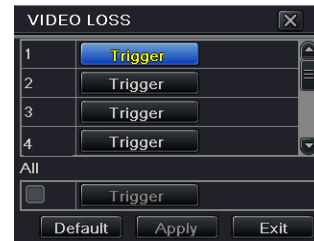
Fig 4-26 alarm configuration-video loss
