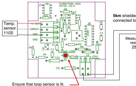
5km shielded cable 2 x 0,5 mm<sup>2</sup>. Shield connected to power supply (-) terminal.
