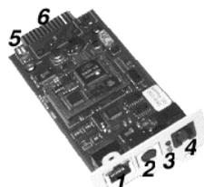
The Internal SNMP-Card can be inserted into an appropriate extension slot of the UPS **POWERNET**. This adapter communicates via the serial port of the UPS and makes a direct multiple server shut down possible without additional SNMP management software.
