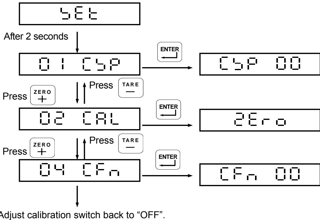
Adjust calibration switch back to “OFF”.
