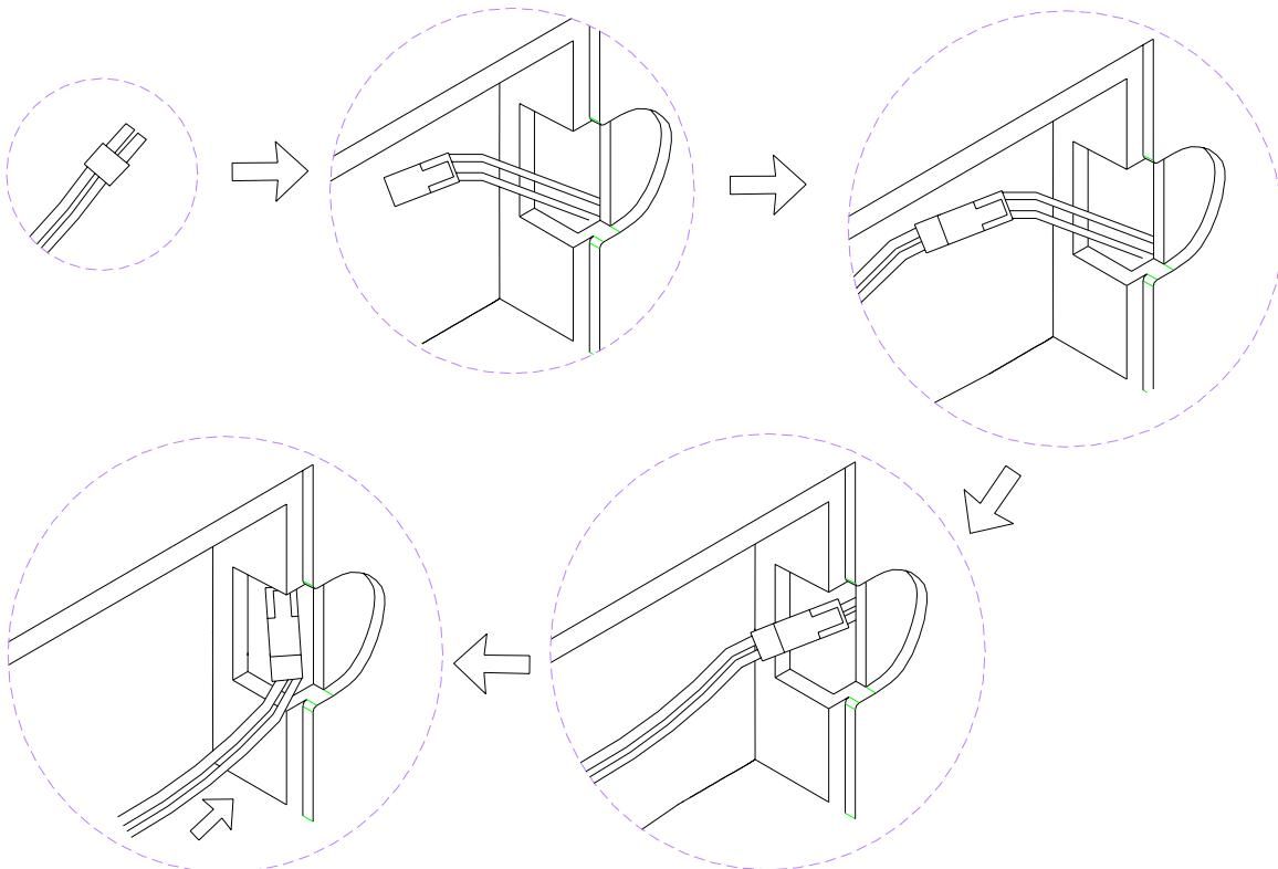
Stuff the surplus wires into the battery case.
