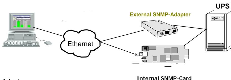
Figure 1.5 SNMP Adapter
