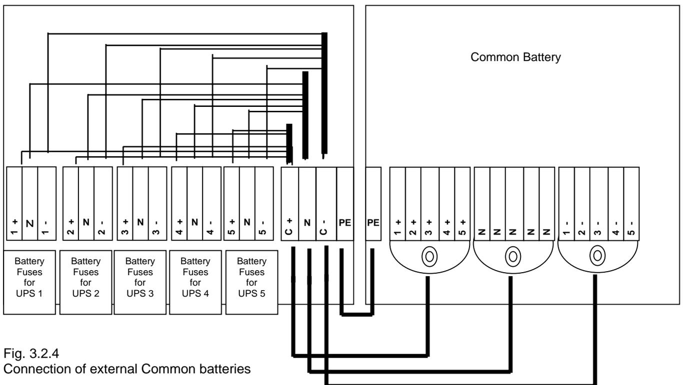
Fig. 3.2.4 Connection of external Common batteries
