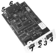
The Internal SNMP-Card can be inserted into an appropriate extension slot of the **PMC**. This adapter communicates via the serial port of the UPS and makes a direct multiple server shut down possible without additional SNMP management software.
