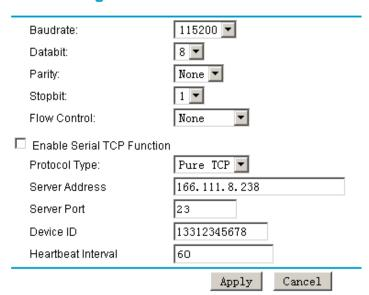
Baudrate: The serial port's baudrate Databit: The serial port's databit
