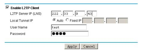
Enable L2TP Client: Enable or disable L2TP Client function L2TP Server IP (LNS): The L2TP server's IP Address
