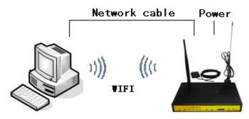
Please modify the IP address of PC as the same network segment address of the router, for instance, 192.168.1.9. Modify the mask code of PC as 255.255.255.0 and set the default gateway of PC as the router's IP address (192.168.1.1).
