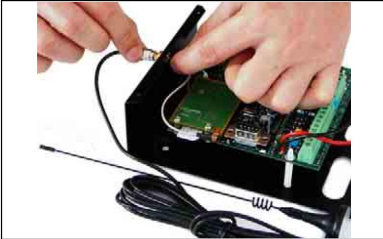
**Figure 14 - Mounting the remote antenna – SmartLink-REM-ANT**
