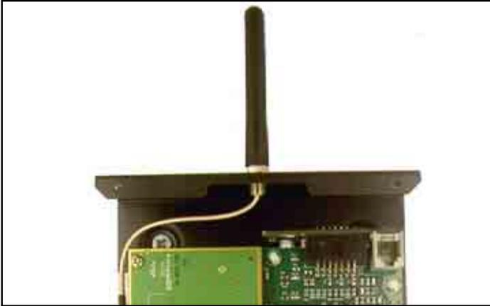
**Figure 13 - Mounting the antenna**
