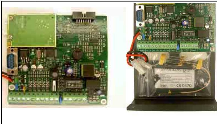
**Figure 6 - SmartLink-GP PCB with antenna**
