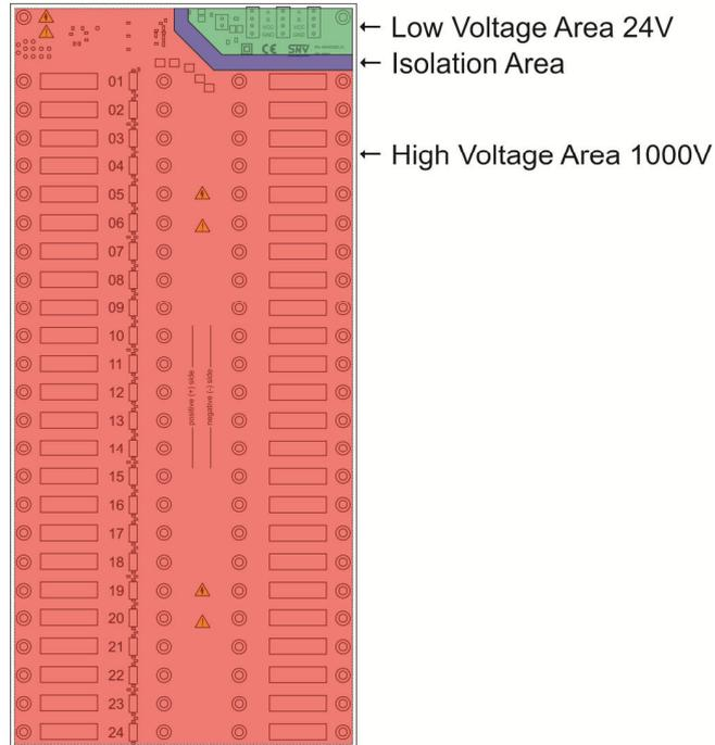
The one (bottom side) is dedicated to the measurement of the current passing through the card and the positive and negative collector bars and to accommodation of the fuses for each string. This area is a high voltage area, where voltage is up to 1000Vdc exist.
