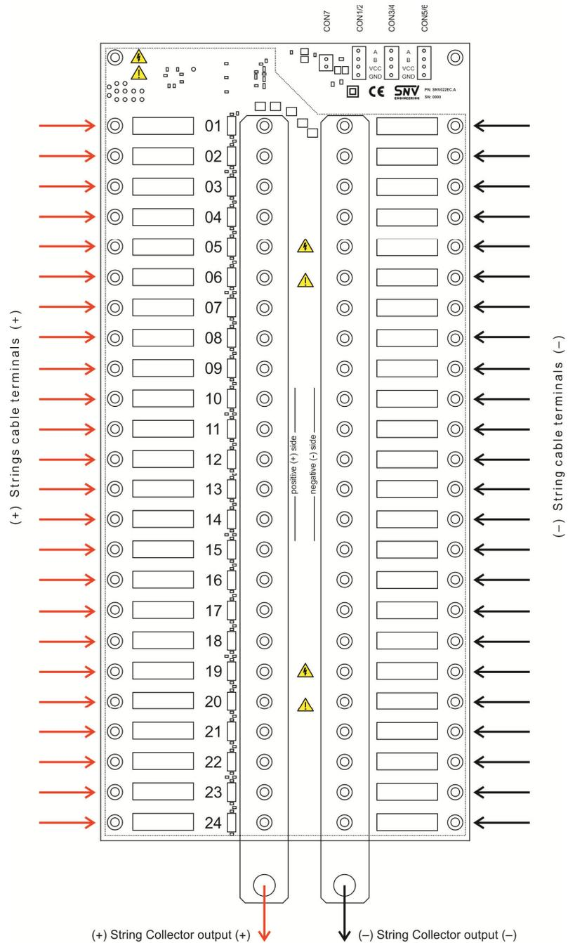
Figure 1: CMC SNV022EC.A Topology Diagram.
