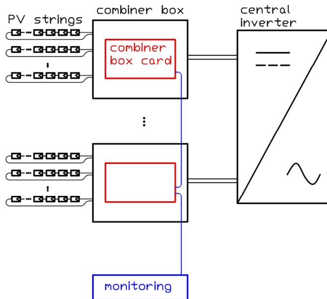
It has on board fuse holder clips for each string for both positive and negative side, avoiding extra cabling and material costs. Current collector bars are premounted and designed to be directly connected to the disconnecter switch for a more clear installation and cost efficient.
