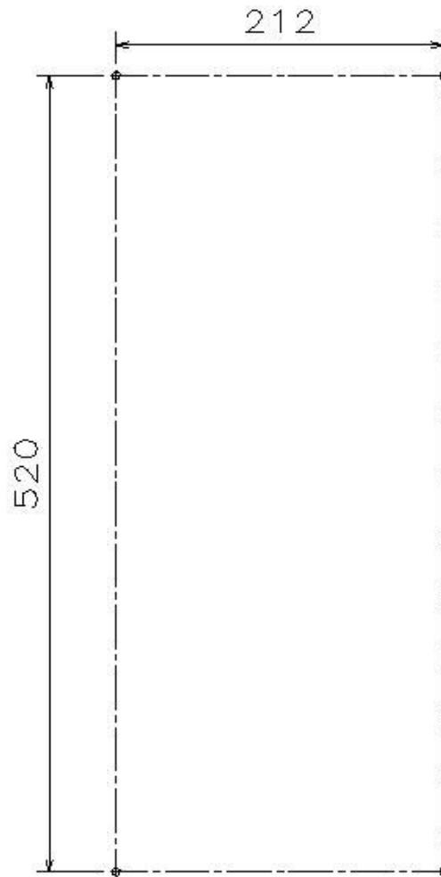
Figure 2: Drilling pattern
