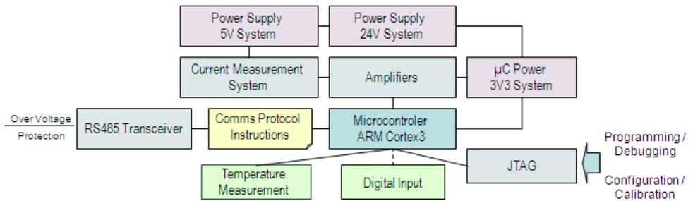
Figure 2: CMC SNV018EC Functional Diagram.
