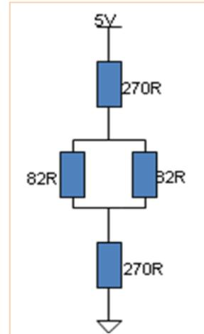
Figure 15: Bus termination and Bias resistors
