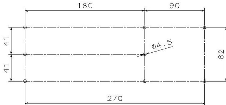
Figure 5: Drilling pattern
