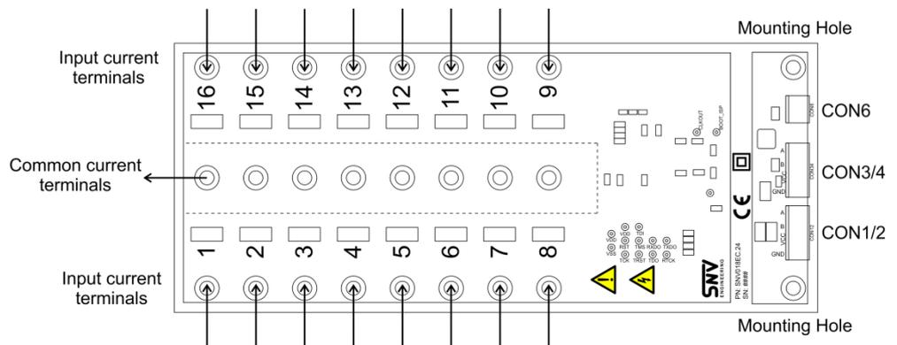
Figure 3: CMC SNV018EC Topology Diagram.
