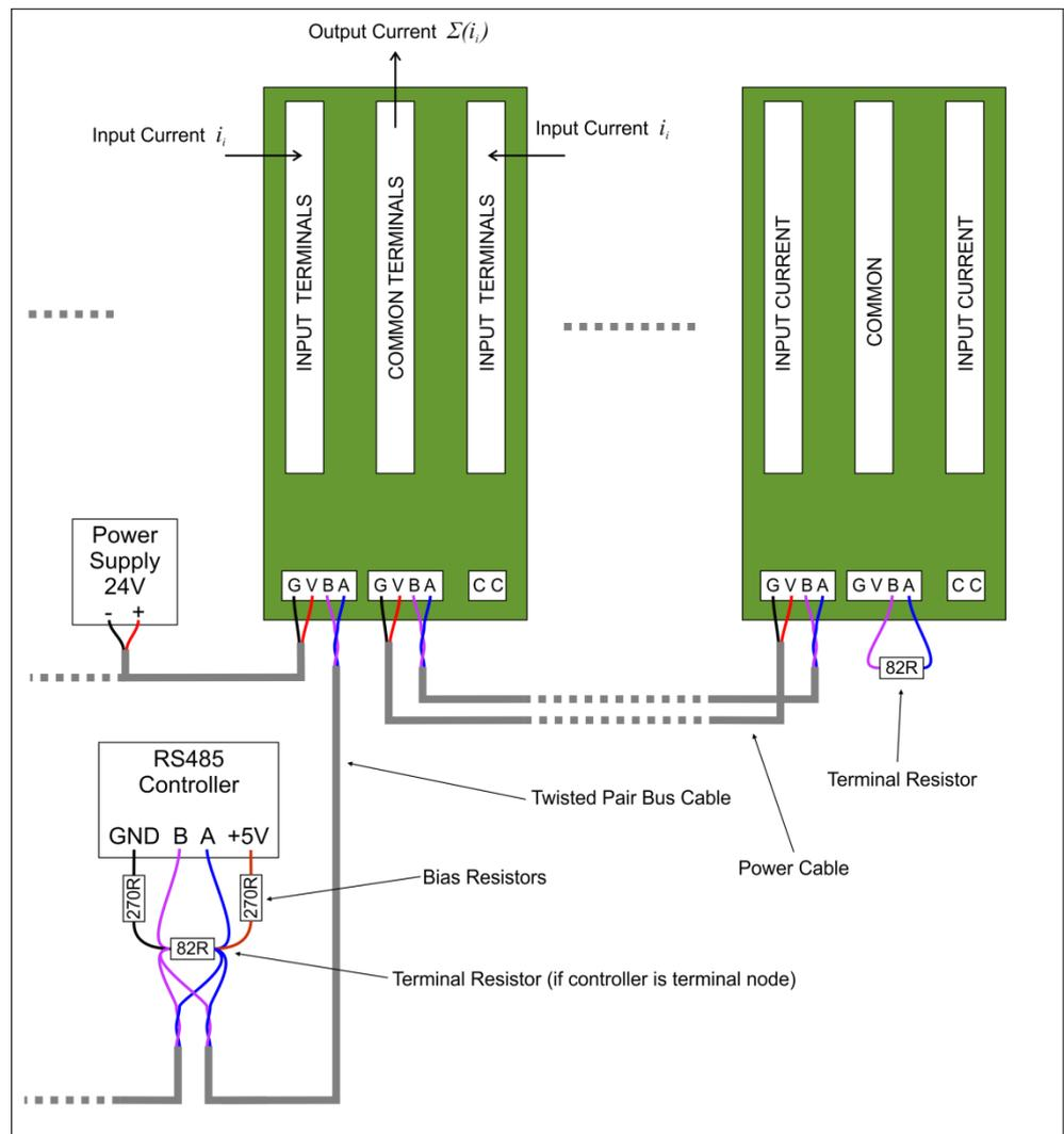
Figure 14: General Bus connection diagram.
