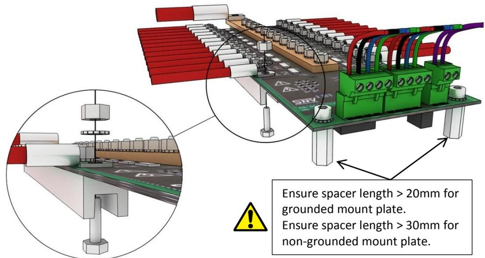
Figure 13: Detail view of "bolt holding bar" mounting
