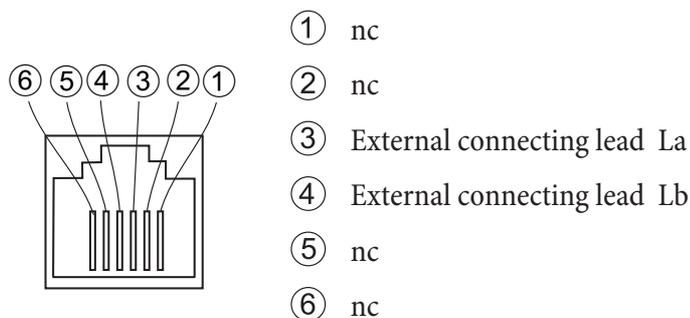
Ports La and Lb are electrically isolated from the PABX system circuit.
