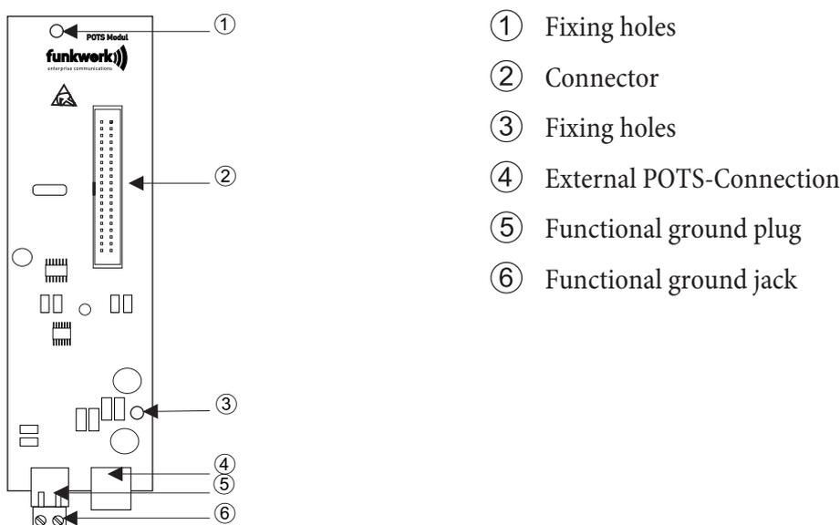
Connection to the PABX system is made using the ribbon cable provided with the system. The external analog port and connection of the functional ground is made using the ports on the module. The marked cut-out areas in the PABX housing must be removed for this. As fine overload protection is integrated into the elmeg M 1 POTS module, function grounding must be connected! The analog port can also be connected via terminals a/b5 / a/b6 to ports la and lb.
