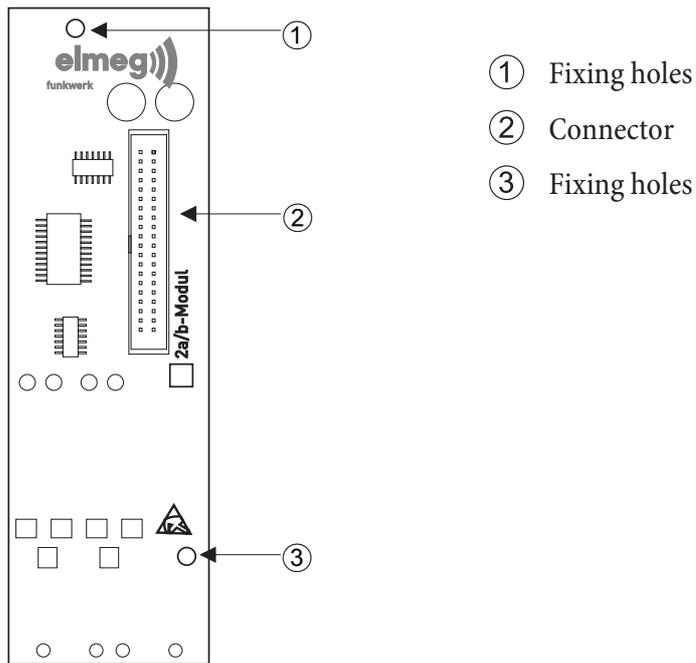
Connection to the PABX system is made using the ribbon cable provided with the system. The two analog subscribers are connected at jacks a/b5 and a/b6 on the PABX system.
