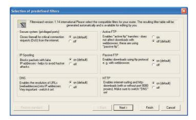
The Filter Wizard can be restarted at any time to load a modified (edited) configuration into the PABX system. Click the button »Send configuration data« to transfer and activate the filters. After the data is sent the new configuration is activated in the PABX system and any ongoing Internet connection is terminated.
