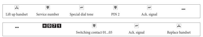
The switching contact closes for the time interval you have programmed (1 ... 999 seconds).
