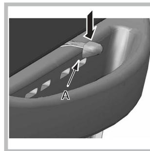
Some models are equipped with a "door lock" device situated between the control panel and the oven door. To open the door, push down device "A" indicated in the figure.
