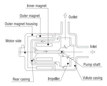
field created between the primary outer magnet and the inner magnet (not visible because housed inside the impeller hub). The magnetic field crosses the plastic parts and the liquid, and firmly couples the two magnet assemblies. When the motor causes the outer magnet to rotate together with its housing, the inner magnet assembly is dragged at the same speed. As a result the impeller, which is integral to it, is maintained in rotation.
