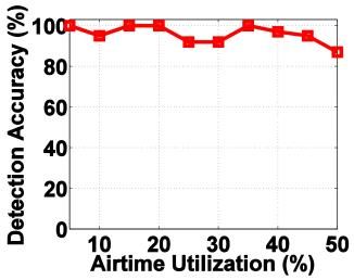
▶ Detection Accuracy > 85% for varying Airtime Utilization of Hidden Link
