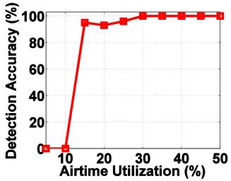
Low Airtime Utilization leads to similar impact as of Hidden Terminal Failure in detection
