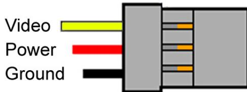
*The power wire is in the center position, so an accidental reverse connection will not cause damage to the device.*
