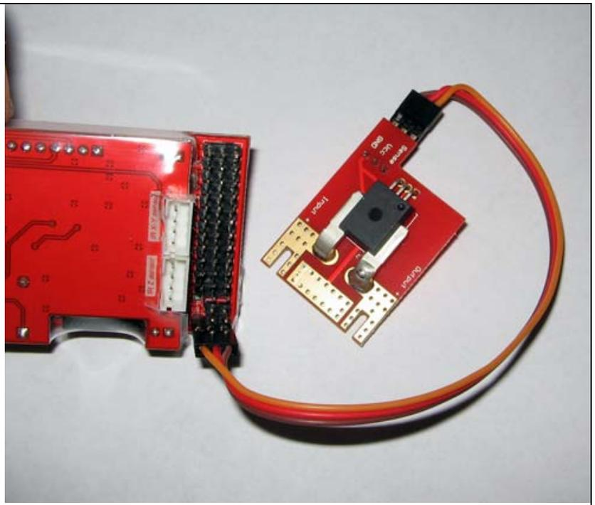
You may use a standard servo extension wire to extend the wire between the RVOSD and current sensor board. Keep in mind the current used by the RVOSD + GPS (150mA) and other devices like the camera and transmitter. Do not use a very thin gauge extension wire.
