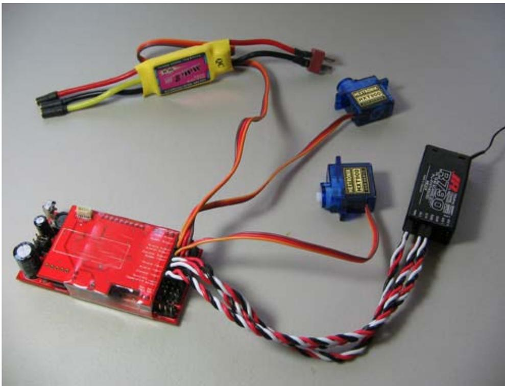
Gen 1 RVOSD shown. Gen 3 has the same type of input/output connections.
