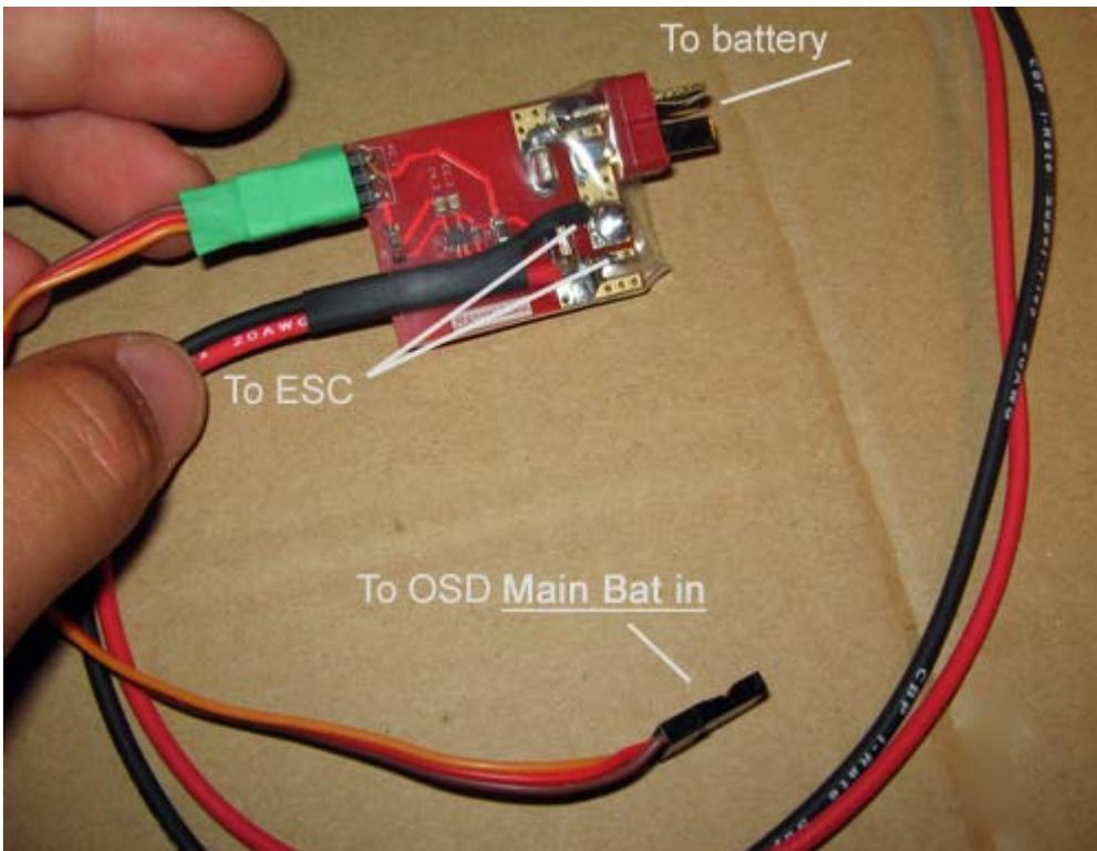
*In this example, I soldered the ESC wire directly to the current sensor board. More reliable and some weight savings.*
