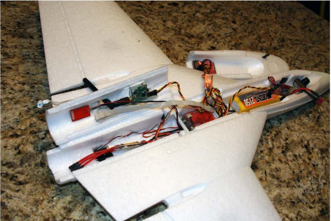
Before making any explanations I will make some suggestions that will save some planes out there. The radio control receiver is very sensitive to electromagnetic fields generated all over the electronics on the plane. Placing your receiver as far as possible from the rest of the electronics (at least 20 cm) is a very good practice. I think the sources of interference can be organized following this order from more to less interfering.
