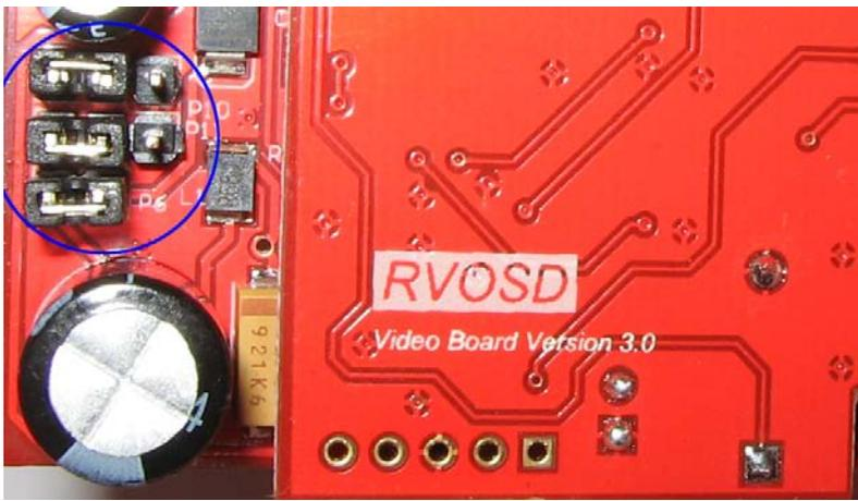
Correct jumper positions for a 12V camera and 12V transmitter, using a 12V main flight battery.
