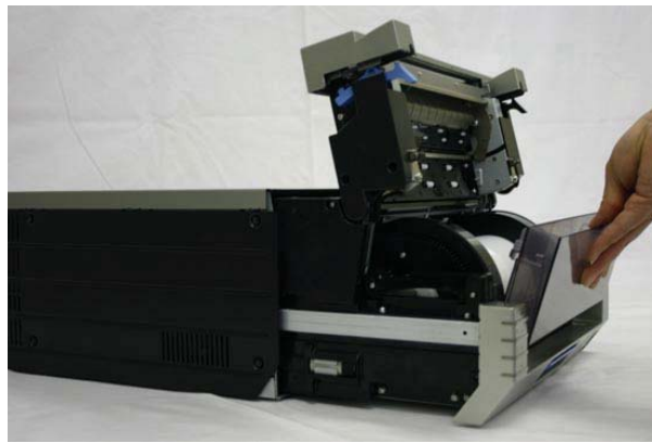
Figure 34. Removing the Scrap Bin
