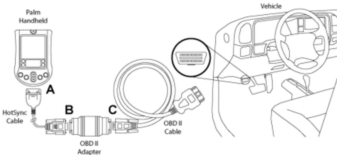
Figure 6: Dyno-Scan™ Connections
