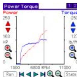
Figure 46: Power vs. Torque Screen
