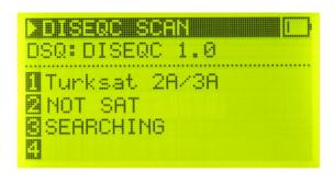
In this menu we may see which satellites are connected to which ports of our Diseq-c Switch. The DISEQ-C 1.0 and Diseqc 1.1 protocols are loaded in your device and are ready to be used. You may use it with all quad and octal Diseqc switches.
