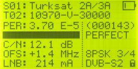
BER / PER : The lower the value of BER in DVB-S1 signals and PER in DVB-S2 signals the better our signal adjustment is.
