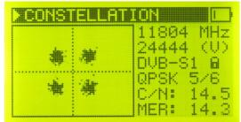
In this menu you may visually see the accuracy of I/Q values after you make the antenna adjustment of the TP and the satellite. When the black points form the smallest circle it means the best adjustment is made. 4 small circles shall form in QPSK signals and 8 in the 8PSK signals. If the signal has not been locked the points will be loose.
