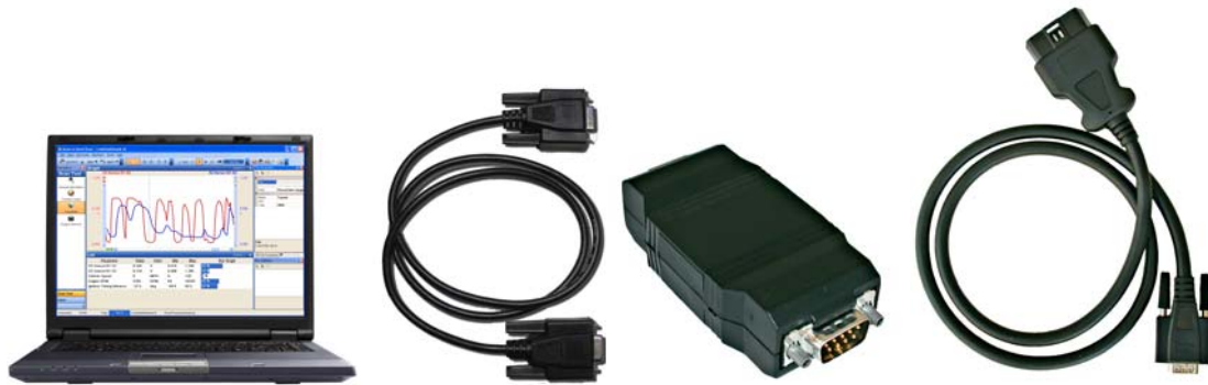
Figure 1: PC, RS-232 cable, OBD II Adapter, and OBD II Vehicle Connect Cable
