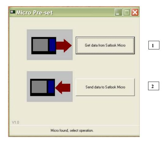
Press the button "Get data from SATLOOK Micro" and this will start the transfer of data. When the transfer is done it will appear a window on the screen for saving this data in a file on the PC.
