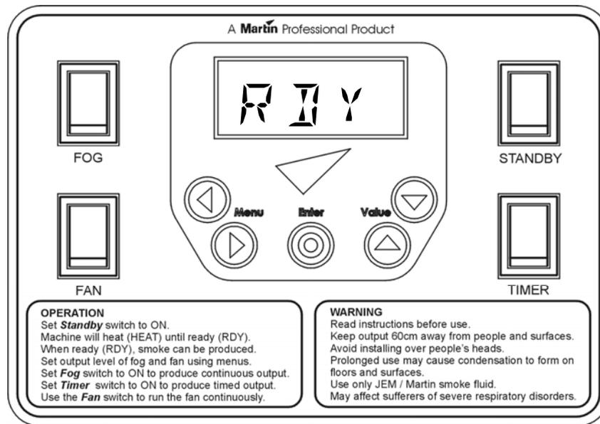
Four **quick access switches** at the sides of the panel allow you to control the main functions:
