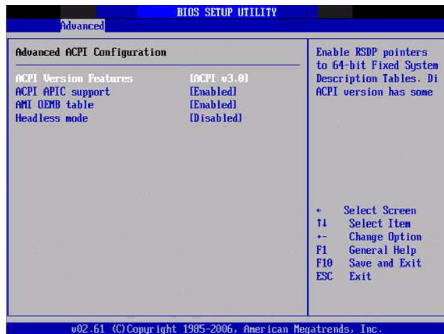
Figure 3.11 Advanced ACPI Configuration
