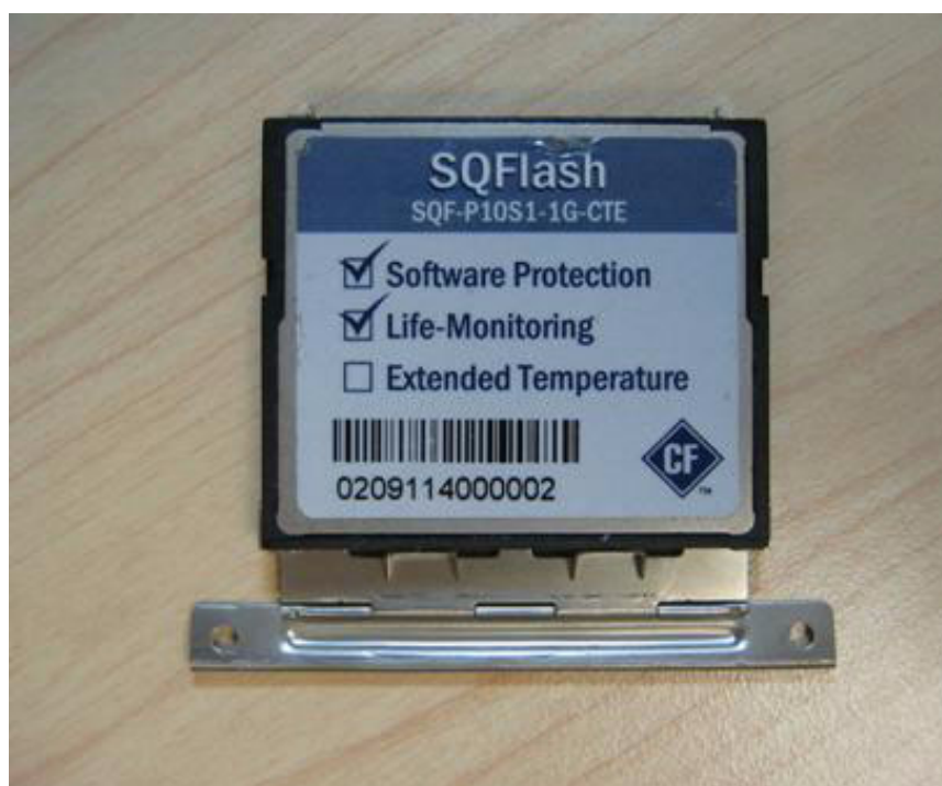
Figure 2.24 Put CF onto the CF tray
