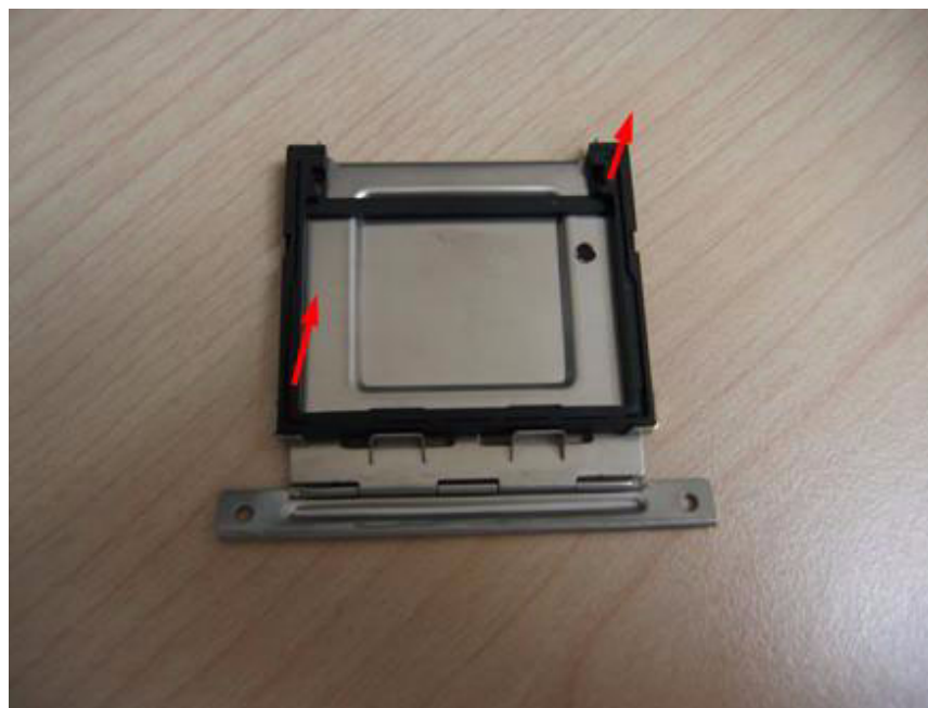
Figure 2.23 Remove CF bracket
