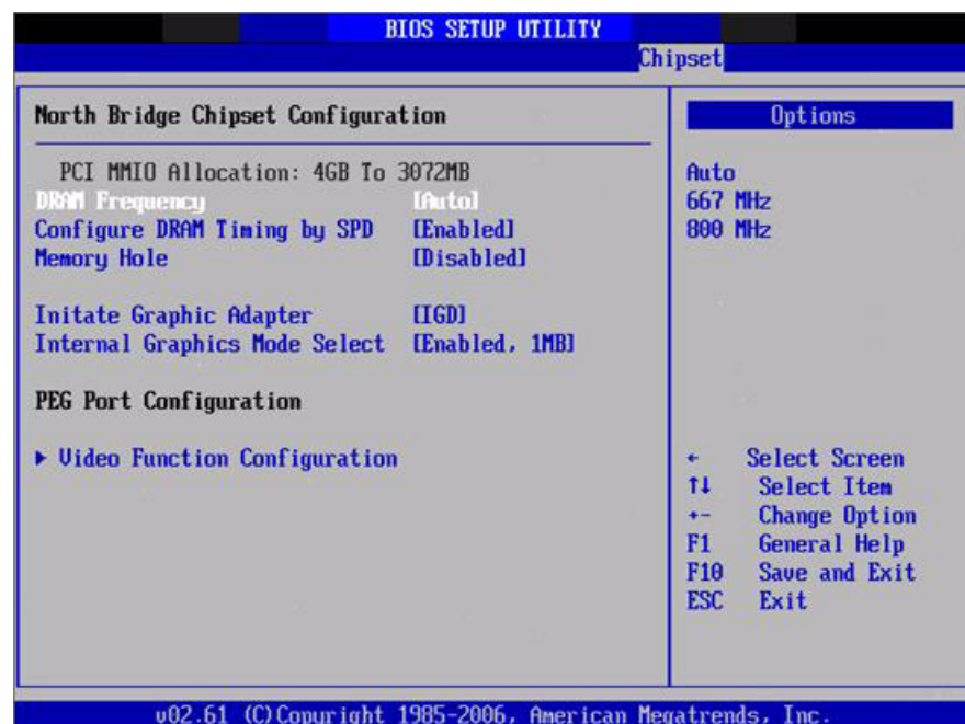
Figure 3.25 North Bridge Configuration
