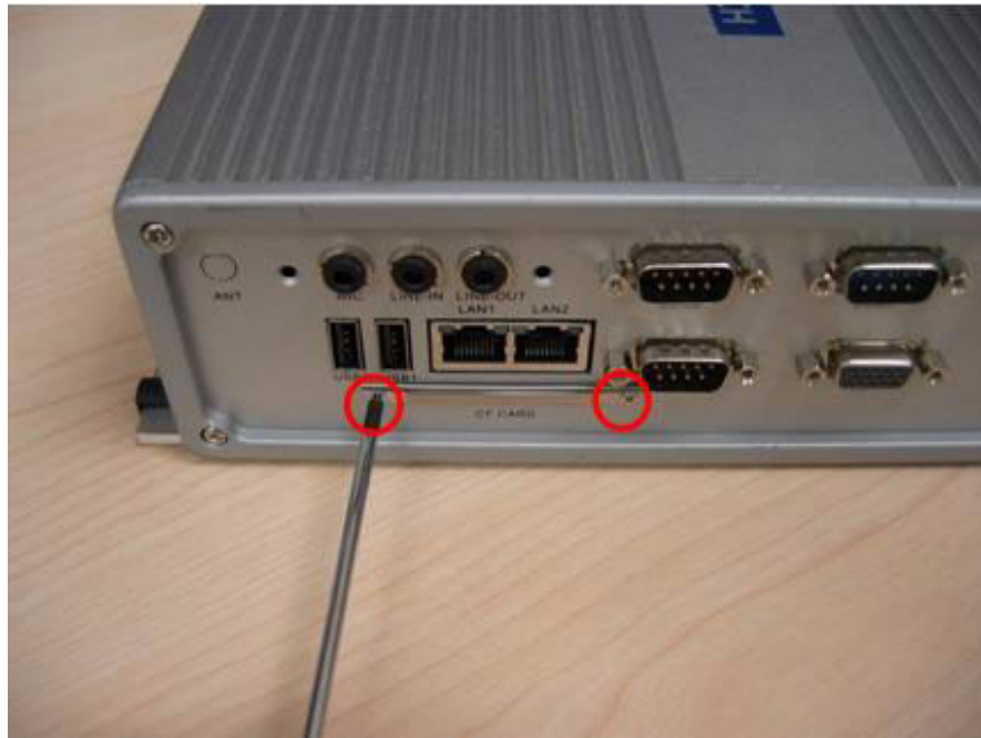
Figure 2.21 Unscrew the CF door screws
