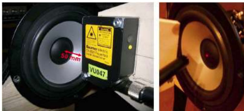
Figure 3.7. Positioning of laser displacement sensor and microphone
