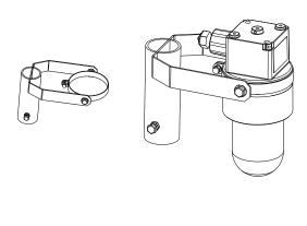
Before opening the housing, unscrewing the assembly of the protective glass, mechanical release should be carried out by unscrewing the blocking screws M4x14 ISO 4027 in the framework of the glass. Removing the lamps is only allowed in the not energized state. Not energized state must be ensured by the exclusion of the voltage at the master switch. It is recommended only to install sources listed in the source table.
