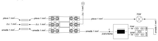
If the user wants to install High pressure sodium source of 50W, it is necessary that the brown phase conductor which is connected to the lampholder E27 is reconnected to the two-pole terminal from 70W to 50W.
