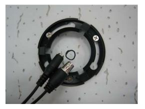
4. Mount the dome body onto the mounting bracket and rotate it until it clicks to secure. Adjust the camera to the correct position and test the dome camera to make sure it is working properly.
