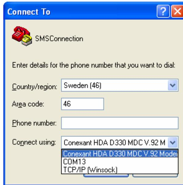
**Figure 3-2 Specifying Serial Port for Mobile Connection**
