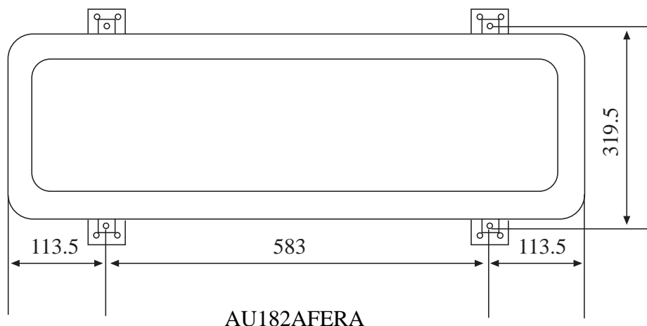
Installation dimension of outdoor unit (mm)
