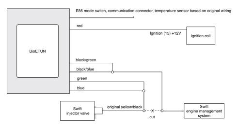
Injector control: from a frontal view, the yellow/black cable for the grey connector on the left side of the central injector. The other yellow cable is the + power for the injector. Warning: do not attempt to use this as the power source for the BioETUN system!
