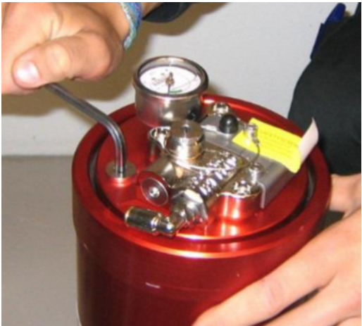
Picture 34. Gently loosen the protection plug
