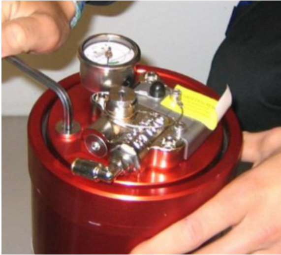
Picture 68. Dismantle the protection plug
