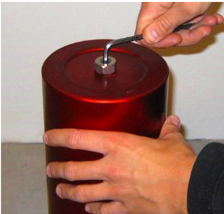
Picture 54. Tighten gas filling screw
