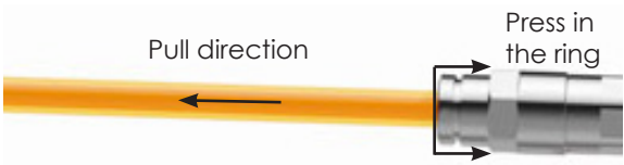
Picture 150. Dismantle coupling from detector tube
