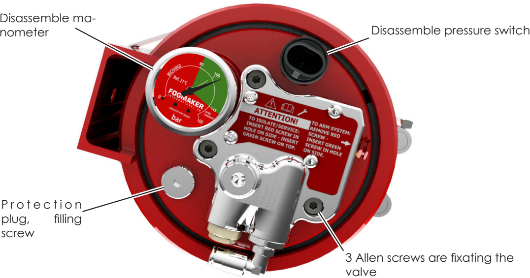
Picture 36. Top view piston accumulator
