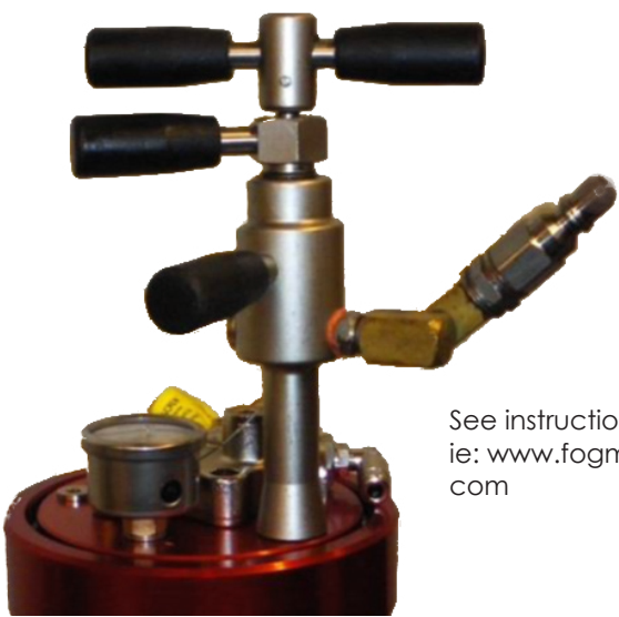
Picture 35. Filling tool mounted on filling screw
