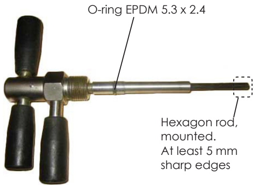
Picture 200. Upper part of filling tool (Part no. 1800)
