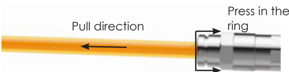
Picture 92. Dismount coupling from detector tube
