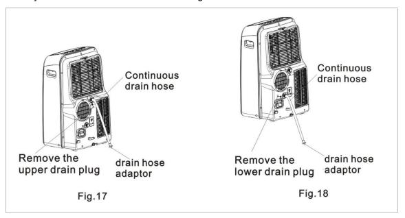
NOTE: Make sure the hose is secure so there are no leaks. Direct the hose toward the drain, making sure that there are no kinks that will stop the water flowing. Place the end of the hose into the drain and make sure the end of the hose is level or down to let the water flow smoothly. Do never let it up.
