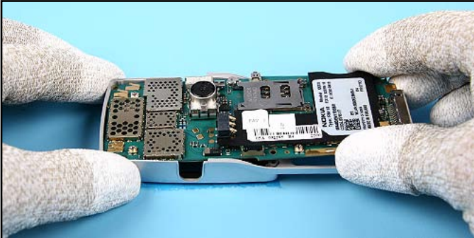
41. Use the A-COVER as a support when removing the CAMERA MODULE.
