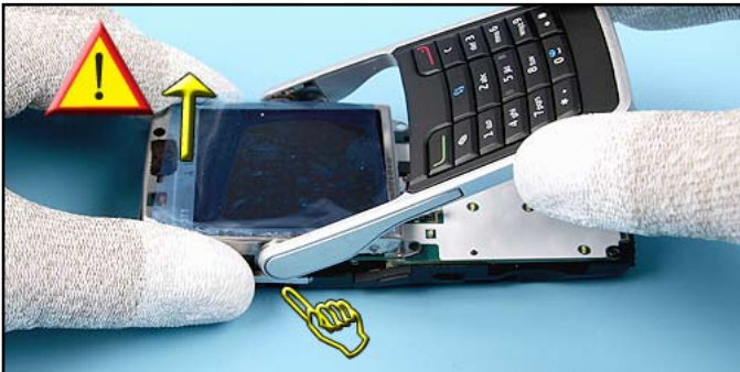
19. Unlock another clip of the FLIP MODULE carefully.
