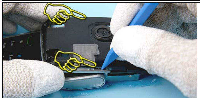
16. The FLIP MODULE is attached to the B-COVER with two snaps.
