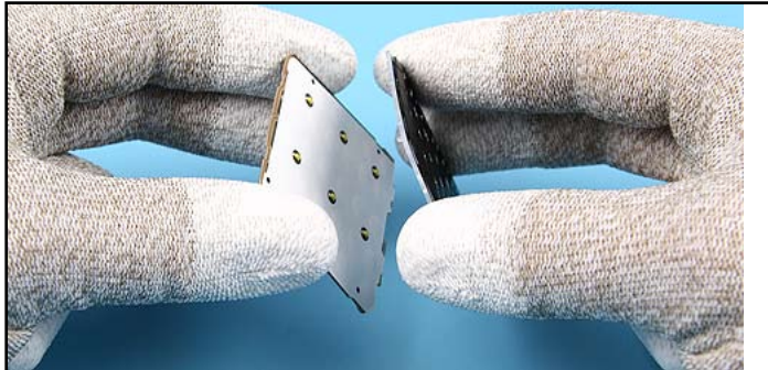
34. Separate the FLIP QWERTY KEYMAT from the FLIP PWB ASSEMBLY
