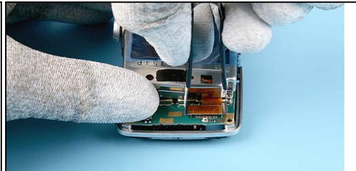
20. Lift the FLIP MODULE a bit and place the flex connector opening tool as shown.
