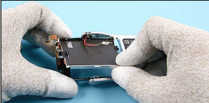
25. Remove the LCD MODULE paying attention to the COAX CABLE.
