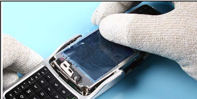
9. Cover the LCD MODULE with a protective film.
