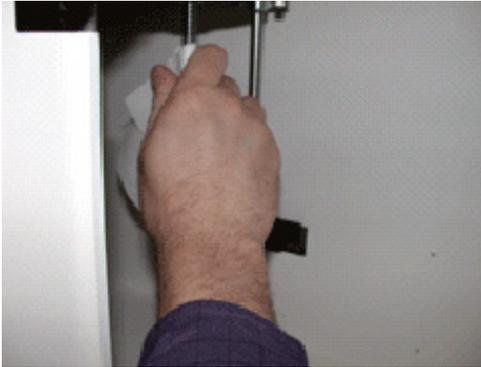
5. Take a paper towel and lightly wipe the feed and build piston screws in order to distribute grease.
