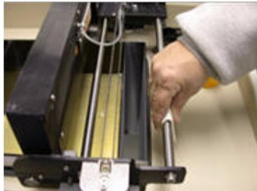
6. Wipe both of the fast axis rails with the paper towel to remove the residue. Make sure to move the carriage and wipe the back of the rail.
