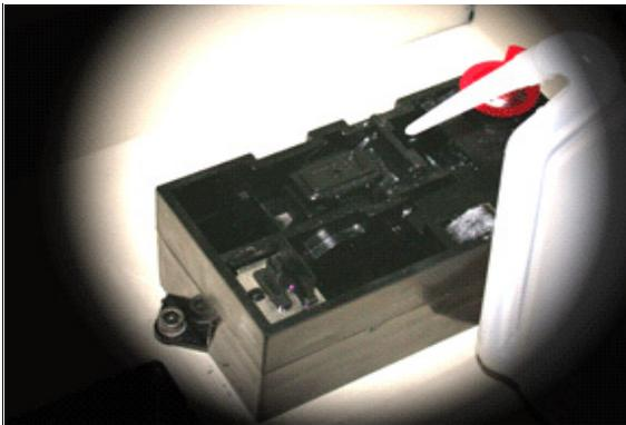
3. Clean and wipe the squeegees and parking cap on the Service Station with distilled water. (See *Section 4.2.6.*)
