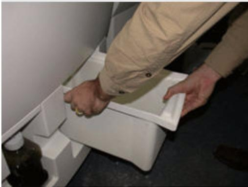
2. Check the overflow bin to see if there is powder to be recycled. If so, remove the powder from the overflow bin and place it in the Feed box.
