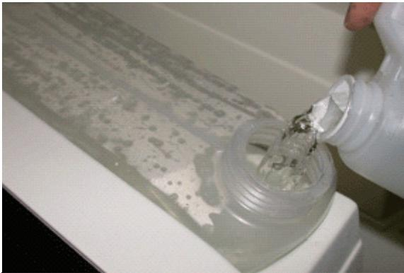
5. Check the binder level and fill if necessary. Fill the binder fluid to the neck of the binder bottle. (See Section 4.2.7.)
