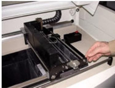
3. Lift the printer top cover and manually move the gantry to expose the Service Station.
