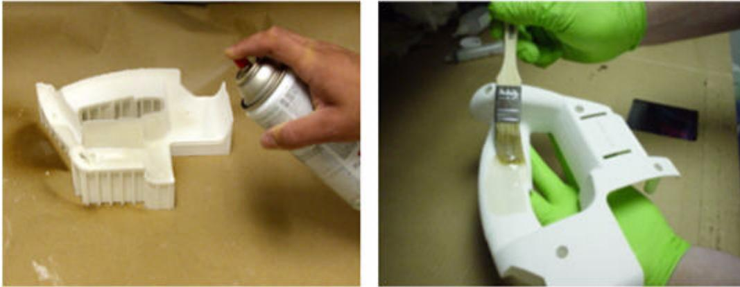
7. Apply Z-Snap epoxy to the rest of the part. Do not apply excess epoxy as pooling will occur. Several thin coats are better than one thick coat. Use a paper towel to remove excess epoxy that may have pooled on the surface of the part.
