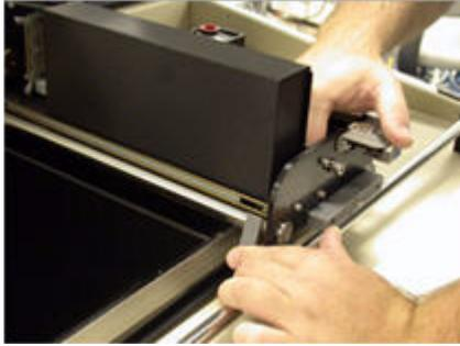
8. Remove the snowplow from the front of the spreader roller. Slide the snowplow away from the edge of the build box until it disengages from the retaining tab. Press on the top edge of the snowplow until it pops off the spreader roller.
