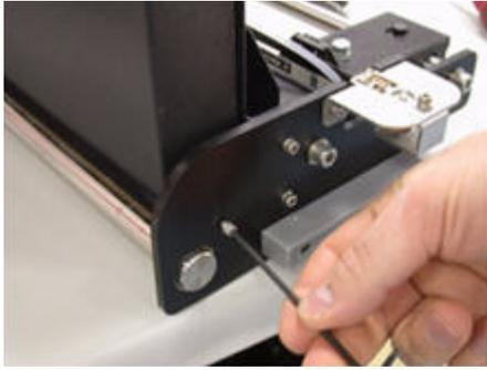
12. Using the 3/32 hex wrench, remove the three hex screws holding the scraper blade retainer and scraper blade onto the printer module.
