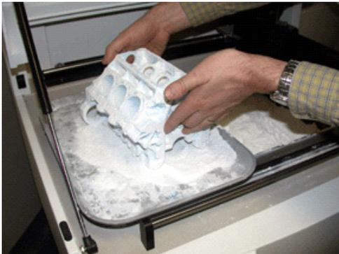
1. Get a tray for transporting the part and place it beside the build box. Use the tools that ship with your printer to remove excess powder from the part. *Gently* remove the part from the build box.
