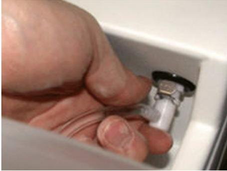
3. Insert the tubing into the latch from the new binder bottle and secure the binder bottle in place on top cover.
