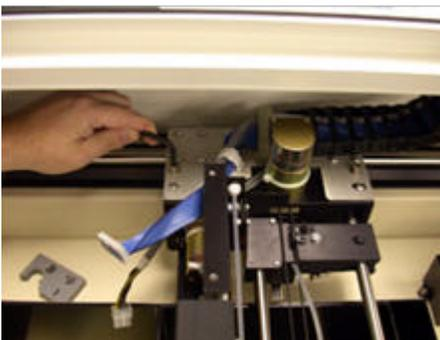
14. Tighten the mounting screws on both sides of the motor assembly.
