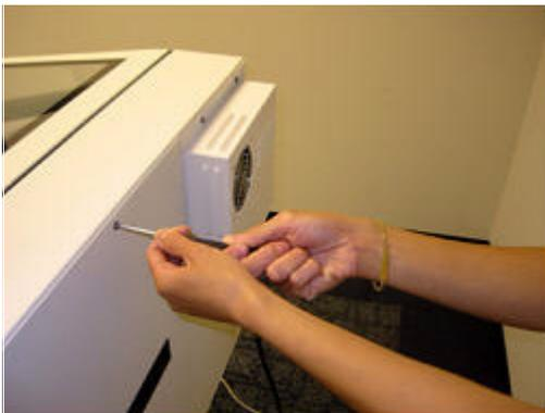
1. If this is the first time greasing the Slow Axis, assemble the grease gun included with the printer toolbox. Follow the instructions on the packaging.
