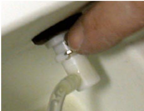
2. Press the release latch and pull the tubing out.
