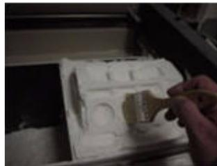
**Stiff Detailing Brush:** This brush has very stiff bristles, which are useful for scrubbing caked powder out of tight areas of a part. The brush is also very helpful when removing fringing from color part surfaces.
