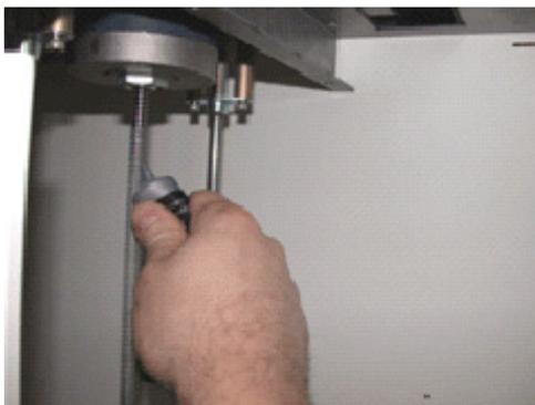
4. Take the grease tube supplied in the Toolkit and apply grease to the entire length of both feed and build piston screws.
