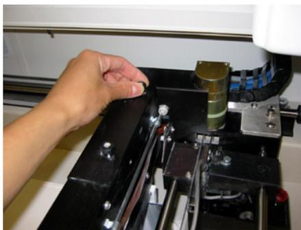
3. Remove the cable enclosure cover by unscrewing the two screws on the top of the enclosure.
