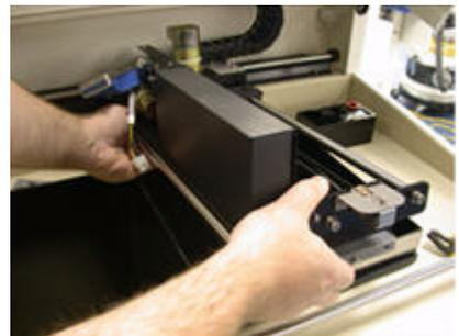
11. Pivot the front of the printer module up while lifting from the rear and remove. Place the printer module on a flat area.
