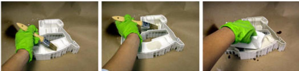
8. Z-Snap parts should sit for 30 minutes at room temperature to allow excess epoxy to drain or wick into the Fixture.
