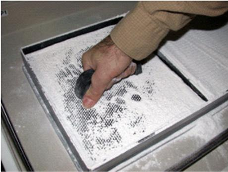
2. When the feed box is filled to the top, take the tamper and slowly press it into the powder surface. Be careful not to “slap” the tamper into the powder, which will produce airborne particles. About 10-15 pounds of force will give it a smooth, flat, and compact surface. Failure to firmly pack the powder will affect part quality.
