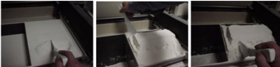
**Soft Horsehair Brush:** This brush has very soft bristles and assists the user with the gross depowdering process. Gently brushing powder away from the part is a useful technique prior to the vacuuming step.
