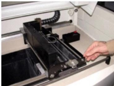
3. Manually move the gantry to the middle of the printer.
