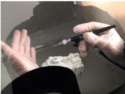
4. Change the air pressure as needed and check the pressure with your hand before applying air to the part.
