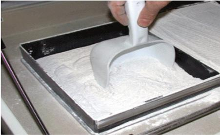
1. Insert the powder scoop repeatedly a few inches into the loose powder to compact it. Continue for about a minute until it feels firm. Repeat for every two scoops of powder.
