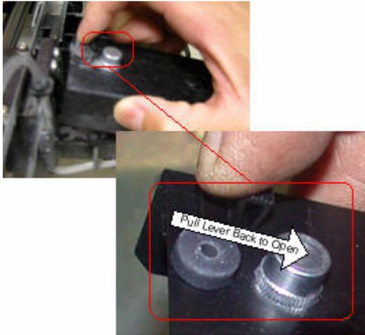
2. Wait for Carriage to unpark, then open the Carriage cover by sliding the latch back to disengage.
