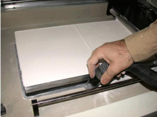
1. Vacuum off any powder that is visible on the printer top deck.
