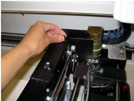
17. Replace the cable enclosure and tighten up the both screws on top of the enclosure.
