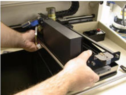
13. Replace the printer module onto the printer.
