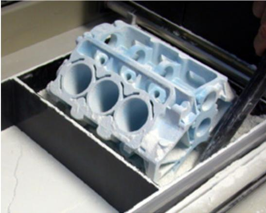
7. At the printer, without raising the build piston, begin vacuuming powder out of the build box. Hold the end of the hose on a 20° to 30° degree angle over the powder so the hose inlet is 1/4" to 3/8" above the surface of the powder. This generates enough of a draft to lift loose powder without damaging the parts.
