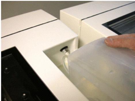
1. Carefully lift and move the binder bottle towards the front of the printer.
