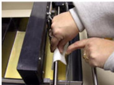
7. To oil the bearings, place the tip of the oil bottle into a fitting. Apply oil for **1 (one) second** to the bearing. Repeat for the second bearing. **DO NOT OVER OIL!** If any excess oil flows out of either fitting, wipe up the excess with a dry paper towel.
