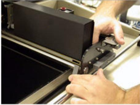
15. Replace the snowplows to the front and back of the roller.
