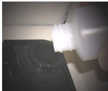
5. Refill the reservoir using the wash fluid supplied in the Toolbox. One bottle will fill up the reservoir. Remember to reorder zc10 Wash Fluid.
