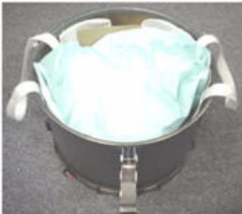
3. Install the vacuum bag inside the vacuum cleaner liner.
