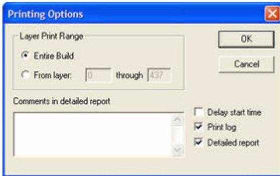
6. Select **File > 3D Print**, or click the **3D** icon on the Toolbar, to initiate the build. The printer will display the **Printing** dialog where the status of the build is reported for the duration of the print. Click **OK** to start the build.
