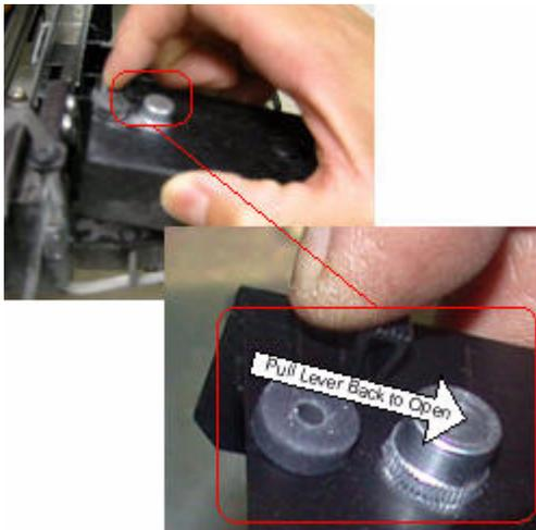
3. Open the Carriage cover to expose the print head.
