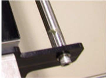
5. Locate any residue buildup on the Fast Axis rails.
