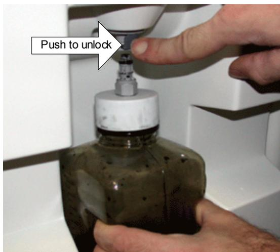
1. Remove the waste bottle by depressing the button on the waste fitting and pulling down on the waste bottle.
