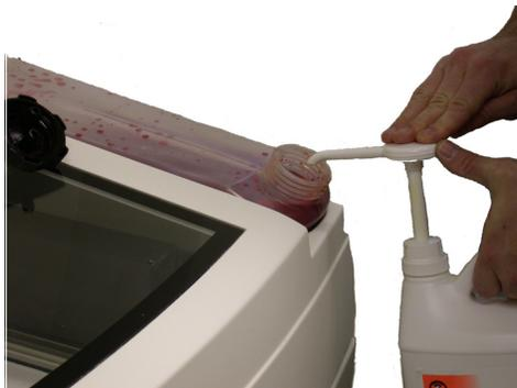
**IMPORTANT:** Higher concentrations of color binder than those stated above will reduce print head life (less than 30 billion pixels). The reduction of print head life will lead to *head over temp* errors and color striping on printed parts.
