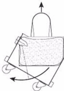
8. Rotate the vacuum canister, in the direction of the inlet, from under the vacuum bag.
