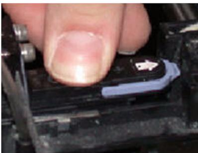
5. Place the new print head in the Carriage and push down to seat the print head. The print head should seat firmly in the Carriage.
