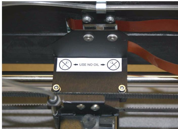
If your carriage has the **USE NO OIL** label, ZPrint will still prompt you to lubricate your printer axis rails. Grease the Slow Axis in the usual way (see *Section 8.8.5*), but **DO NOT** oil the Fast Axis. To close the dialog, click **Dismiss**. When the prompt “*Did you lube Axis Rails?*” appears, click **Yes** to close the prompt to reset the maintenance counters.
