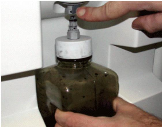
6. Check the waste bottle. Remove and dispose of liquid in accordance with local disposal regulations. (See Section 4.2.9.)
