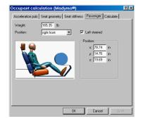
If "Left Steered" is checked (default), the steering wheel will appear for the Left Front seated position. If unchecked, the steering wheel will appear for the Right Front seated position. The occupant's seat position is the occupant's H point in the vehicle coordinate system, as measured from the front center of the vehicle at ground level.
