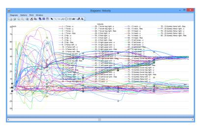
In order to view individual graphs clearly, it is possible to turn some of them off. This is done by selecting  $\langle Options \rangle \langle Diagrams/Axis \rangle$  in the "Diagrams" window. This opens a window in which each item has a check box beside it. Click on each check box to turn it off or on.
