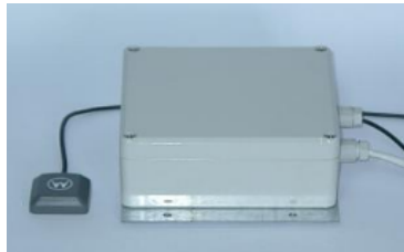
Figure 4: NTS-3000 GPS antenna and converter box
