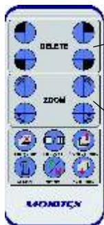
**Delete:** Press shaded quadrant to delete the specific image from the quadrant. Press "Freeze" to re-capture image for the quadrant.
