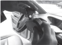
1. Attach the mounting bracket to the main unit
