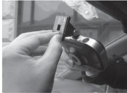
2. Place the unit on the installation point (windshield) and remove the red film from the tape on the mount
