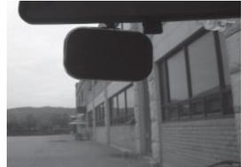
3. Install the unit on the upper & center on the windshield as shown above
