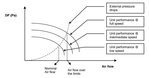
In the EC fans the rotation speeds are selected with different values of the control tension (0 - 10V). The right value of the control tension has to be set by keyboard, considering the AESP requested on site. If the unit is equipped with the "air flow control" option, the mp manage the fan speed in order to obtain the required air flow (Air flow set-point).
