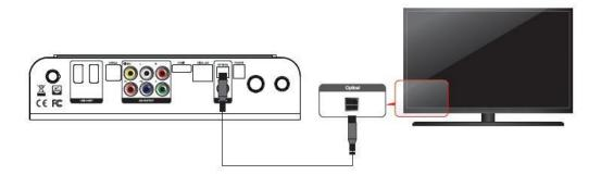
You can enjoy high-quality 5.1CH sound when connected to an amplifier or a receiver with optical cable. Connect optical cable to Optical port on Xtreamer Prodigy as shown above. Then, connect to an amplifier or a receiver. (Optical cable is optional)
