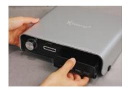
**01.** Open the hard disk cover on the front panel
