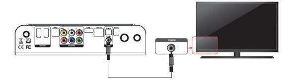
You can enjoy high-quality 5.1CH sound when connected to an amplifier or a receiver with coaxial output cable. Connect coaxial cable to coaxial port on Xtreamer Prodigy as shown above. Then, connect to an amplifier or a receiver. (Coaxial cable is optional)
