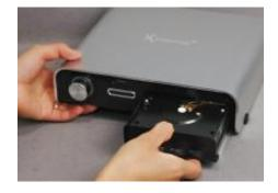
**03.** As shown here, slowly and carefully push the HDD guard together with the HDD into the main body of Xtreamer Prodigy.
