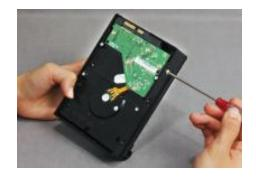
**02.** Connect the HDD guard to an HDD as shown on the picture. Fasten the screws.
