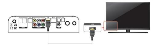
Connect HDMI cable to HDMI terminal at the back of product. Connect the remaining cable terminal to HDMI terminal at the back of a digital TV. Make sure to carefully distinguish between input and output terminals.
