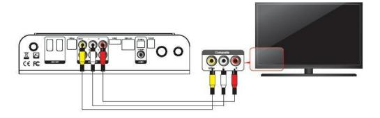
Connect yellow cable for video signal to the terminal located at the back of side of TV. Then, select external input of TV. Connect the remaining red and white terminal cables to the left/ right and audio output terminal at the back of the device. Then, connect red and white cables to the left/ right terminal of DTV input or component audio input located at the back of a digital TV.
