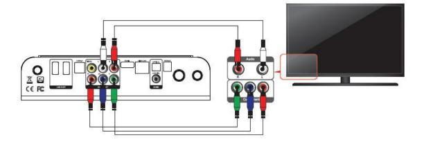
Connect the green, blue and red terminal cables to the Xtreamer Prodigy and TV in accordance with the color scheme; connect white AV cable to L terminal, and red AV cable to R terminal. (Component cable is an optional item)
