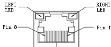
The network status LED indicator on the RJ45 socket
