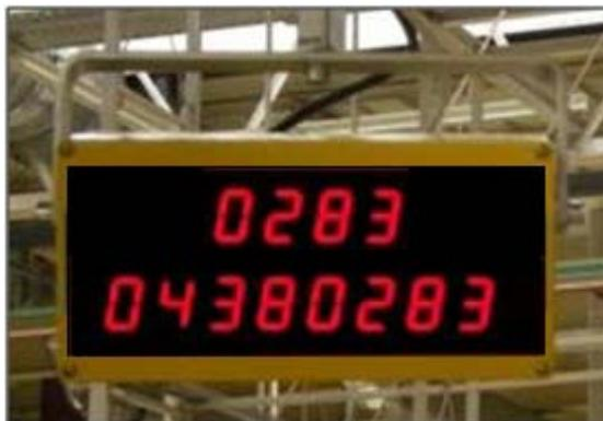
Its purpose is to display the identification number of the product/unit that is currently located at the workstation (8 digits) and the sequence number (4 digits).
