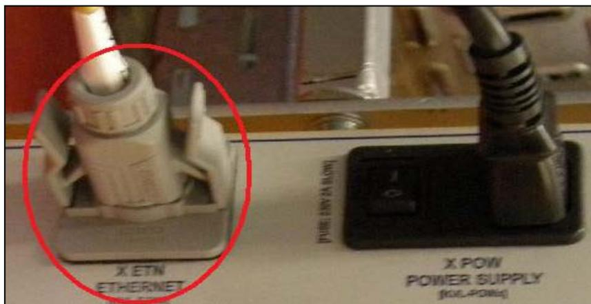
The industrial Ethernet socket is of type VARIOSUB-RJ45.
