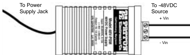
Figure 10: Connecting DC Power to the 2701/I DC Power Supply.
