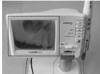
**Step 4.** The image of X-Ray film shows on the LCD monitor after push the film cassette in.
