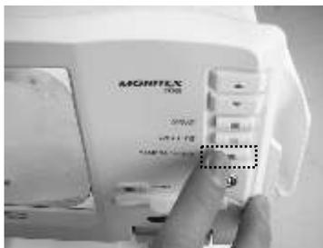
**Step 2:** Press CAMERA/X-RAY button to switch to Intraoral Camera mode.
