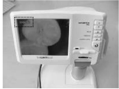
**Picture Code:** For each saved images in the Micro SD card, there are numbers coded and appearing on the monitor. This picture code can be used to retrieve for download.
