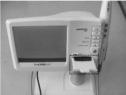
**Step 3.** Place the X-Ray film into the Plastic cassette.
