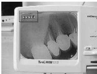
**Number Code:** The images that saved inside the SD card are coded in numbers which appear on the screen.
