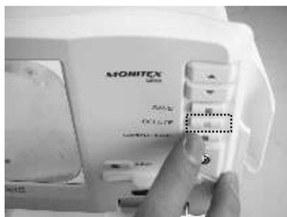
**DELETE Image Step-2:** After the image is selected, press DELETE to remove it from the SD card.
